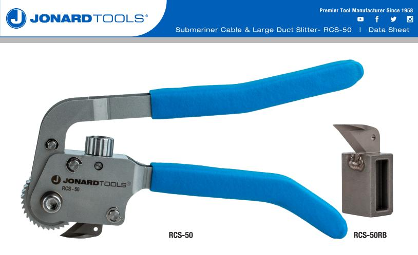
Designed to open the toughest heavy-duty cable and duct jackets, the RCS-50 is perfect for performing lateral and longitudinal cuts on submariner cables, large fiber ducts, or large count telephone cables at least 1 1/2" (3.81 cm) in diameter. This ratcheting cable slitter also features the following:
