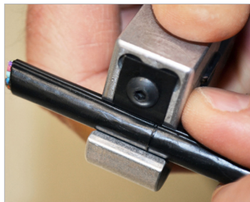
Precision ripping blade performs longitudinal cuts by slitting along the ridge of the cable jacket.
