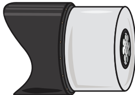
STRIPPING SEMI-CON FROM URD CABLE
